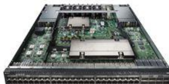
P4 programmable switches
